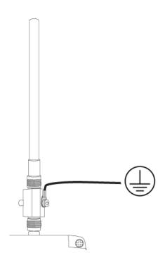
Figure 28. Grounding for Antenna
