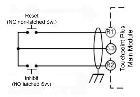
Figure 18. Optional Remote Reset and Inhibit Switch Connections.
