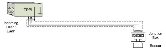
Figure 27. Grounding for Screened Cable with Plastic Junction Box and Sensor
