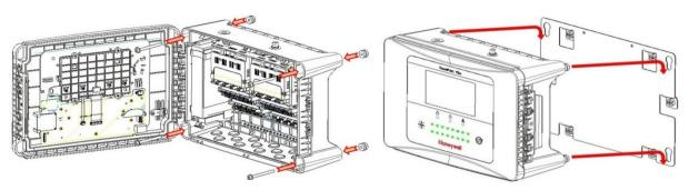
Figure 13. Wall Mounting Plate Option
