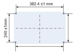
Figure 12. Wall Mounting Points
