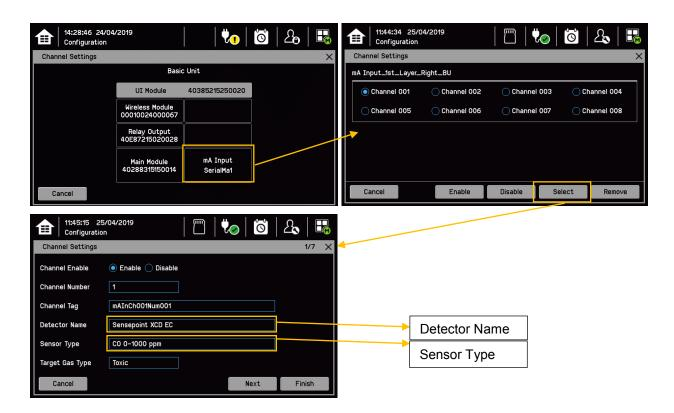
**Note**: Refer to Ch.14 Configurable Parameter Reference Guide for the list of available detectors. You can also use the TPPL Sensor Catalog to select listed gases, or you can enter 'User gas' details if respective gas is not listed.
