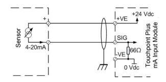
Figure 21. Two Wire Device Powered by a mA Input Module
