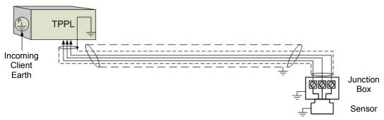
Figure 24. Grounding for Screened Cable with Armour and with Metal Junction Box and Sensor
