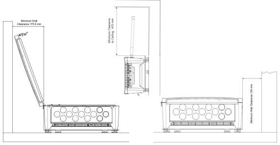
Figure 11. Installation Clearance Measurements
