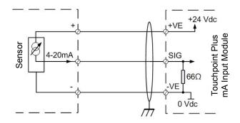
Figure 19. Three Wire Device Powered by a mA Input Module
