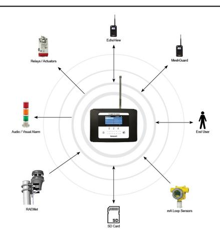
Figure 7. Typical Installation Options
