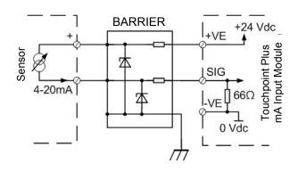
Figure 23. Two Wire Device Barrier Device Powered by a mA Input Module
