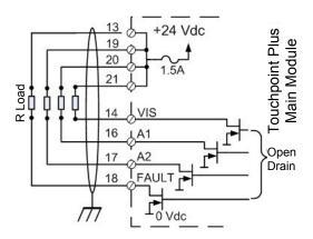
Figure 17. Dedicated Alarm Circuit Connections
