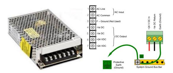
**Note:** Mains Earth (Ground) must only be connected to the protective earth (ground) rail, and not to the SMPS.
