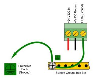
Figure 16. Connections for DC 24 V Supply
