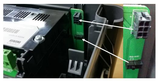
Figure 37. Battery On/Off Switch and Battery Connector
