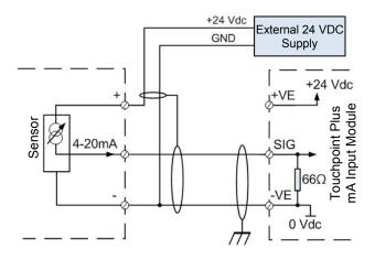
Figure 20. Three Wire Device Powered by an External Source
