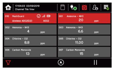
The screen will display a list of the input channels with active Alarms, starting with the most recent event. Unacknowledged alarms will flash, acknowledged ones will be stay on. Touch the Accept button to acknowledge the alarms.
