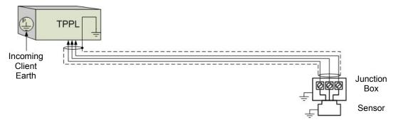
Figure 25. Grounding for Screened Cable, No Armour, with Metal Junction Box and Sensor
