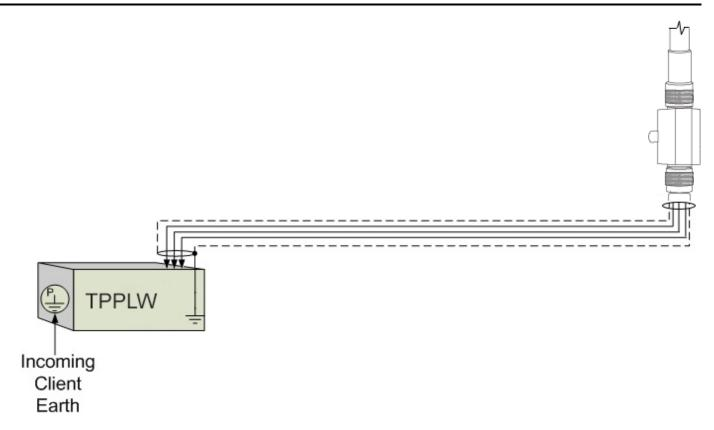
Figure 29. Grounding for Antenna Extension
