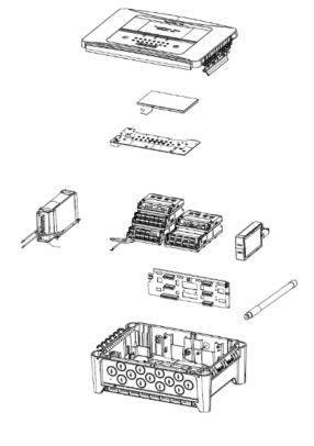
Figure 8. Controller Exploded View
