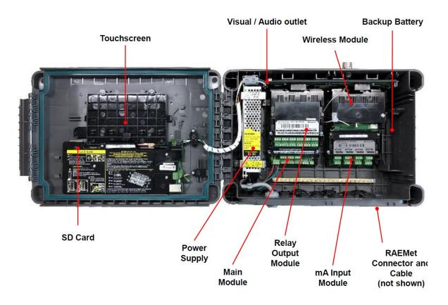
Figure 9. System Layout Before Installation
