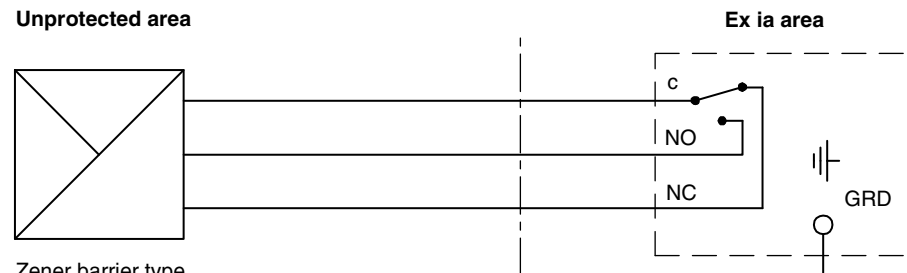
Fig. 6: Operation of pressure switches in intrinsically safe areas
