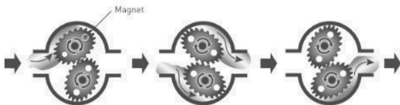
Figure 1 Schematic oval gear operation
