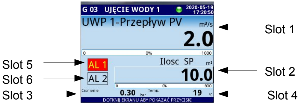
Fig. 7.160. Slots layout in controllers view
