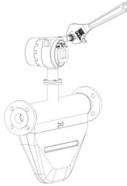
Fig.4.5 The installation of power cable
