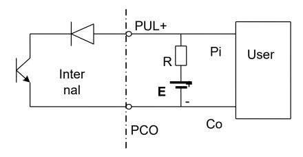
Fig 2.7 Digital Output Direct
