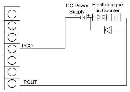
Fig 2.5 (a) Example of electromagnetic counter
