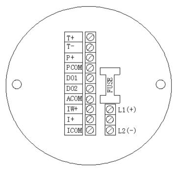
Fig 2.2(b) Compact Type: Terminals and Marks
