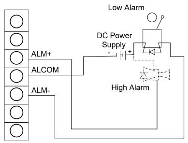
Fig 2.5 (c) Example of alarm output
