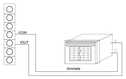
Fig 2.4 Wiring of current
