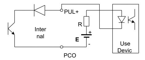
Fig 2.8 Connection with photo-coupler (e.g.
