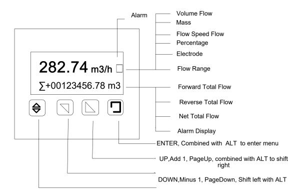
Fig 2.1 (a) Remote Type: Keypad and LCD
