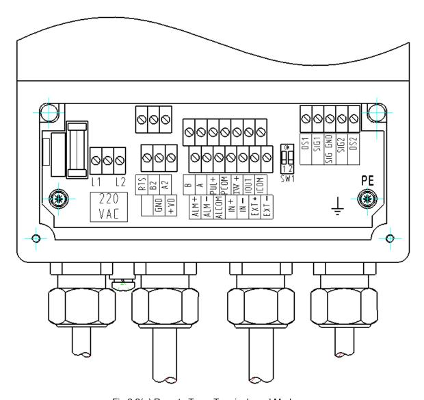
Fig 2.2(a) Remote Type: Terminals and Marks
