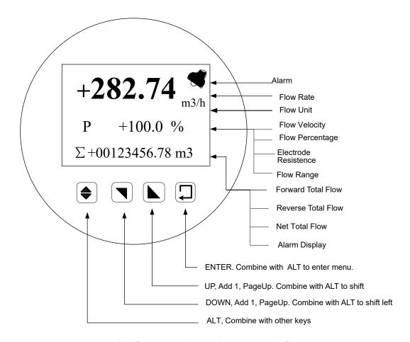
Fig 2.1(b) Compact Type: Keypad and LCD
