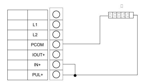
Fig 2.5 (b) Example of electrical counter
