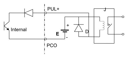
Fig 2.9 Connection with relay (e.g.
